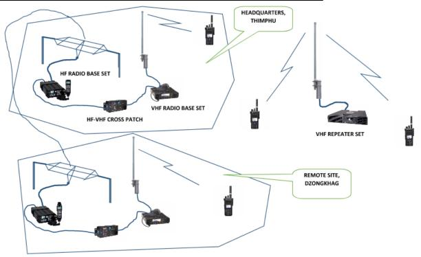
5. Besides the existing 14 VHF repeater stations, five additional new VHF repeater stations have to be installed at the Microwave stations of Bhutan Telecom. Therefore, there are 19 VHF repeater stations in total spread across the country. These repeater stations will be used for local communication, between Gewog to Dzongkhag or Dzongkhag to Headquarters depending on coverage. The detail of location of repeater stations with rough coverage is as tabulated below:-
